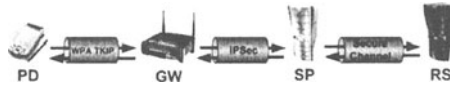
Fig. 6. In a secure network, packets must only travel through encrypted and authenticated channels.
